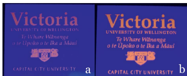
Figure 10. Comparison between images printed using 1 layer (a) and 2 layers (b) of ZnS:Mn 2+ quantum dots.
