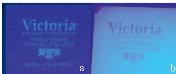
Figure 11. A detailed inkjet-printed image of the Victoria University of Wellington logo on photographic-quality inkjet paper using ZnS:Cu 2+ quantum dots (a), and on cotton fabric using ZnS:Mn 2+ quantum dots (b).
